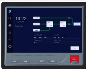
Color touch screen display with integrated 4 channel oscilloscope for troubleshooting input, output, and DC signal without any use of special software or encrypted tools. Allows analysis of 3 phase voltage, current, frequency, DC link voltage and DC current within the UPS chassis.
